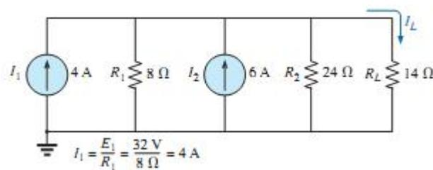
$$I_s = I_1 + I_2 = 4 \text{ A} + 6 \text{ A} = 10 \text{ A}$$
