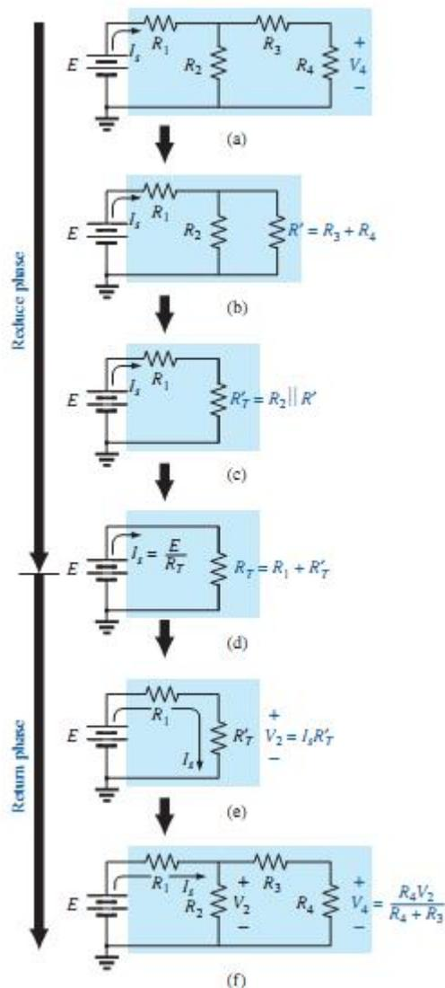
Example : Find current  $I_3$  for the series-parallel network in Fig. below.
