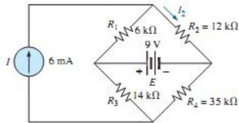
Solution: Considering the effect of the  $6\text{ mA}$  current source
