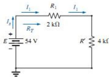
Substituting the parallel equivalent resistance for resistors  $R_2$  and  $R_3$
