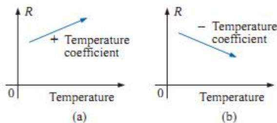
it is important that we have some method of determining the resistance at any temperature within operating limits. At two different temperatures,  $T_1$  and  $T_2$ , the resistance of copper is
