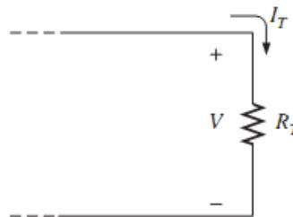
The current  $I_T$  can then be determined using Ohm's law:
