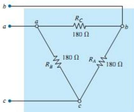
Example : Find the total resistance of the network in Fig. where  $R_A = 3\Omega$  ,  $R_B = 3\Omega$  , and  $R_C = 6\Omega$  .
