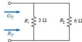
**EXAMPLE :** Determine the effect on the total conductance and resistance of the network of previous Fig. if another resistor of 10  $\Omega$  were added in parallel with the other elements.
