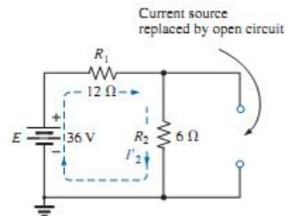
$$I''_2 = \frac{R_1(I)}{R_1 + R_2} = \frac{(12 \Omega)(9 \text{ A})}{12 \Omega + 6 \Omega} = 6 \text{ A}$$
