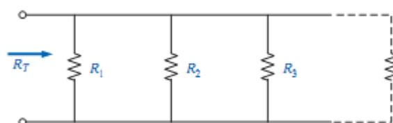
Determining the total resistance of parallel resistors.
