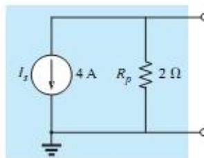
EXAMPLE : Reduce the network in Fig. below to a single current source, and calculate the current through  $R_L$  .
