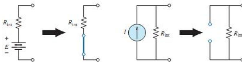
Since the effect of each source will be determined independently, the number of networks to be analyzed will equal the number of sources.
