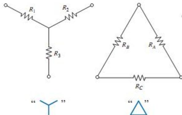
The purpose of this section is to develop the equations for converting from Δ to Y, or vice versa.
