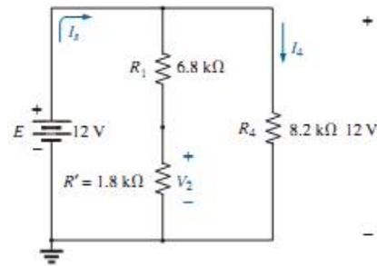
H.W// Determine all the currents and voltages of the network in Fig. below.
