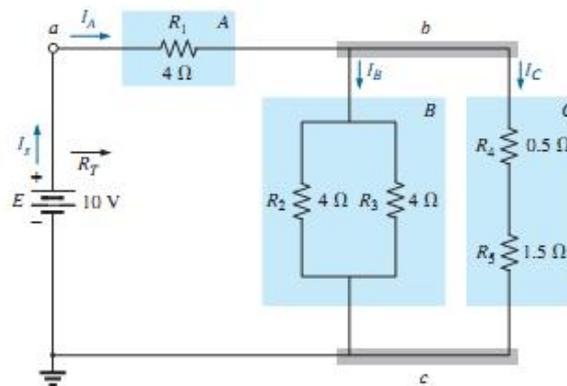
H.W// Find the indicated currents and voltages for the network in Fig.
