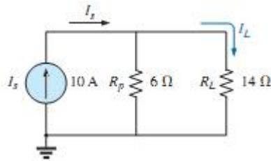
$$I_L = \frac{R_p I_s}{R_p + R_L} = \frac{(6\ \Omega)(10\ \text{A})}{6\ \Omega + 14\ \Omega} = \frac{60\ \text{A}}{20} = 3\ \text{A}$$
