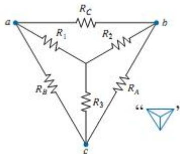
$$R_1 = \frac{R_B R_C}{R_A + R_B + R_C}$$
