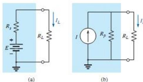
the load  $R_L$  would not know which source it was connected to. This type of equivalence is established using the equations appearing in Fig. below. First note that the resistance is the same in each configuration a nice advantage. For the voltage source equivalent, the voltage is determined by a simple application of Ohm's law to the current source  $E = IR_p$ . For the current source equivalent, the current is again determined by applying Ohm's law to the voltage source:
