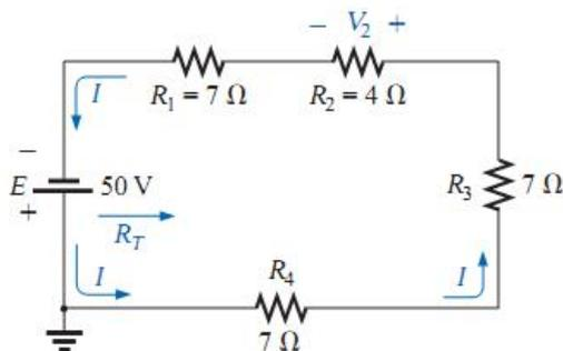
Solution: Note the current direction as established by the battery and the polarity of the voltage drops across  $R_2$  as determined by the current direction. Since
